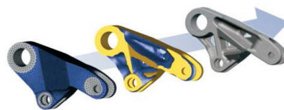
Topology optimization of a lever (Images courtesy of JCB)
